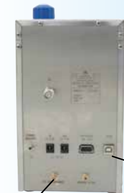
BOECO LAC-SA with 2 peristaltic pumps inside, 1 for cleaning, 1 for sample
