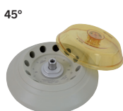
Angle rotor, 12-place Cat. No. 01252-A 12-place, n = 14,000 min -1 , max RCF 15,558
