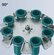
Swing-out rotor, 8-place, n= 4,000 min -1 , max. RCF 2,415, for 8 x 15 ml, stainless steel, with suspensions No. 01644, PA, fibreglass reinforced.
