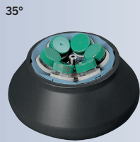
Angle rotor, Cat. No. 01556 6-place, n= 9,000 min -1 , max. RCF 10,595
