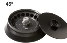
Angle rotor, Cat. No. 01627 18-place, with bioseal, phenol-resistant lid n= 14,150 min -1 , RCF 22.161, for 5 ml microtest tubes
