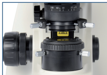
KOEHLER ILLUMINATION / SLIDING-IN ABBE BRIGHT FIELD CONDENSER
