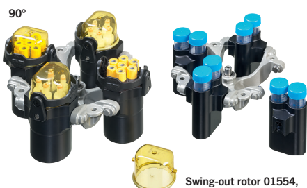
Swing-out rotor, 01554, 4-place, illustrated with carrier 01560 and lids 01561 n= 4,500 min -1 , max. RCF 3,328 for max. 4 x 200 ml
