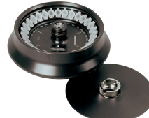
Angle rotor, Cat. No. 01553 30-place, incl. bioseal lid, phenol resistant n = 14,150 \text{ min}^{-1} max RCF 21,713
