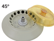
Angle rotor, 18-place, Cat. No. 01258-A n = 14,000 min -1 , max RCF 16,654
