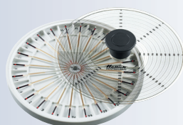
Haematocrit rotor with lid as evaluation disc included.
