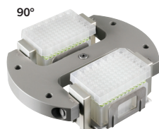
Swing-out rotor, 2-place, n=4,000 min -1 , RCF 2,218 for microtitre plates, aluminium, coated, with suspensions No. 01453-A, stainless steel.
